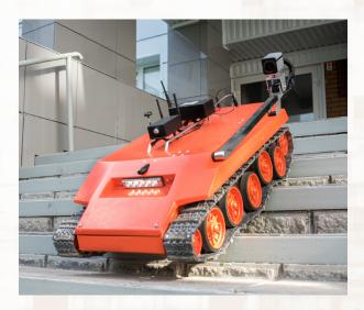
The system consists of the following elements: universal control station, robotic platform of the increased cross-country capacity, chassis cameras, high-resolution camera with 24x optical zoom, night vision camera (thermal imager, gamma-locator, high-radiation resistant camera), ASMRCS (automated system for monitoring radiation and chemical safety), directional auto tracking antenna, sweeper units, clamshells.
